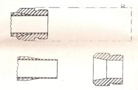
The straight turning and the taper can be accomplished at one operation by setting the lathe compound at 10°. The straight part can then be turned with the carriage and the taper with the compound. Polish the exposed portion of the tube with fine abrasive cloth.
